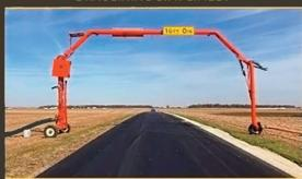
Now manure applicators can cross a road wherever is convenient for them, and not be forced to find a culvert to run the hose under the road.
