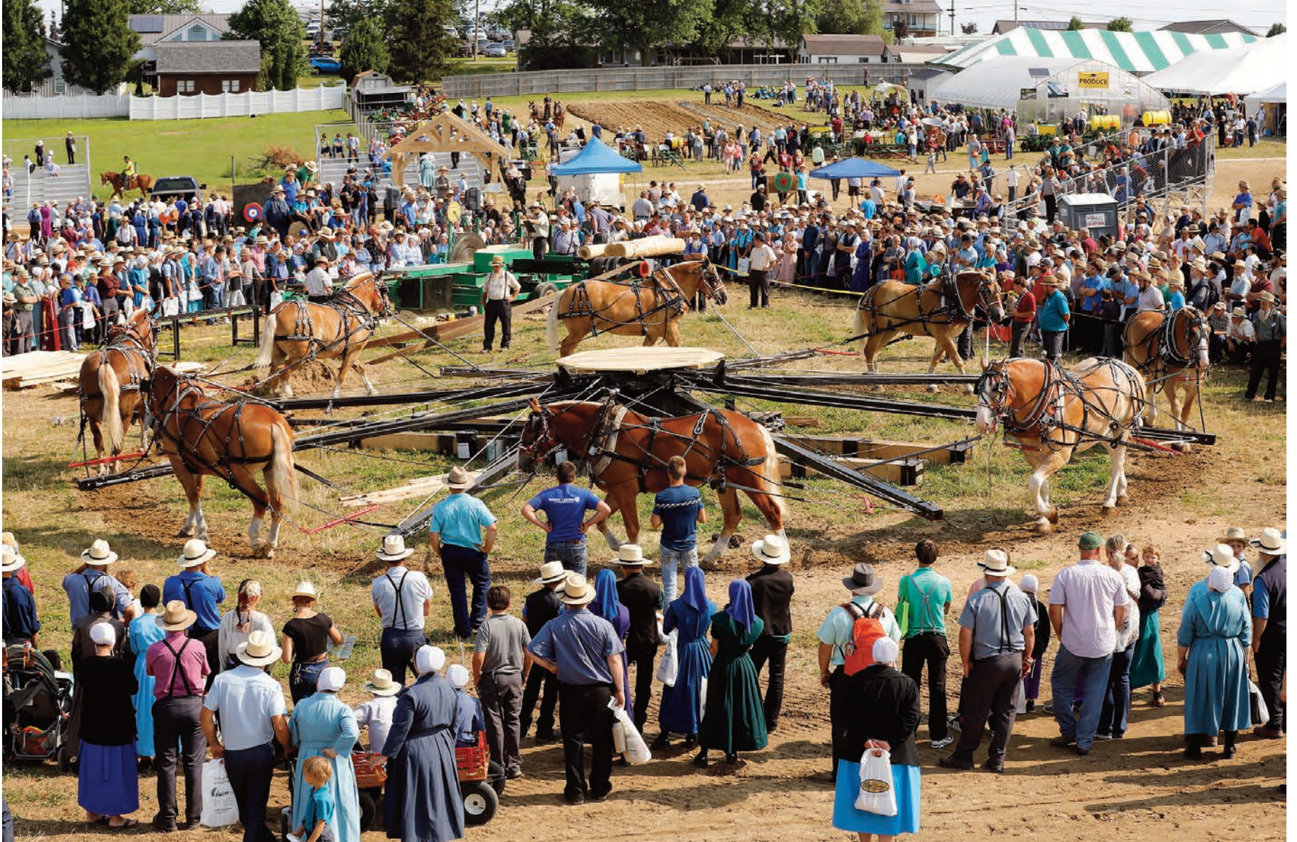
Pictured are eight Belgian horses hitched to a sweep as they walk in a circle. The central gearbox powers a horizontal shaft with a pulley on the end belted to a sawmill. This picture was captured at the 2021 Horse Progress Days in Mount Hope, Ohio. As shown, crowds gathered in great numbers to view the unique operation. Photo by Lynn Telleen, Draft Horse Journal
