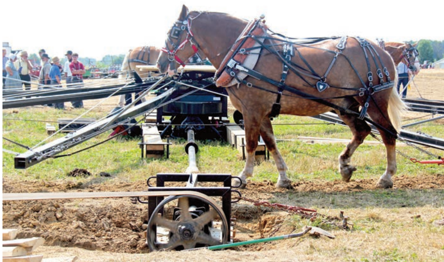
This view shows the horizontal shaft with the pulley belted to a sawmill. The arms to which the horses are connected to the gearbox are shown with stabilizing cables. The shaft end is slightly above ground so the horses must step over it. Photo by Fred Hendricks
